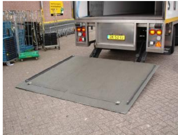
Tail-lifts with polyurea coating
