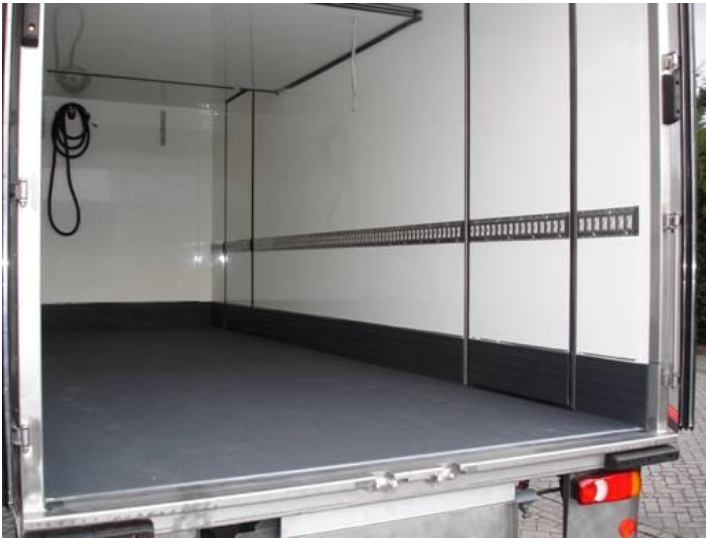
Floors with polyurea coating
