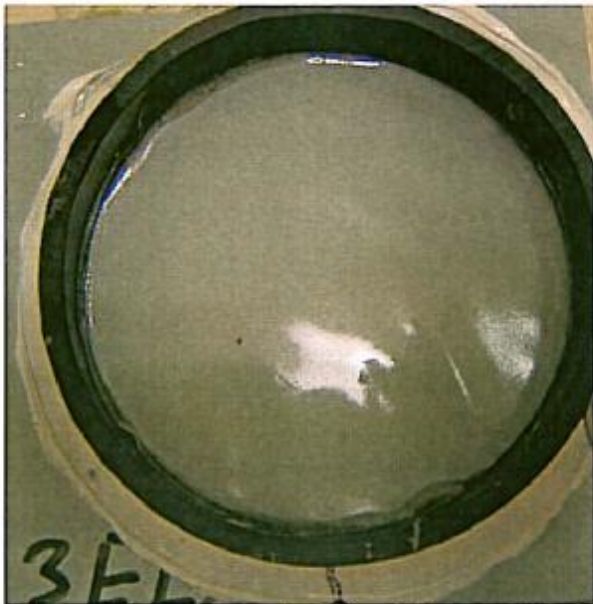
Figure 7: One sample after 7 days subjection to 20% ammonium hydroxide
